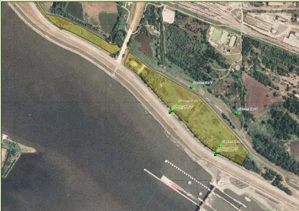
Figure EA-3. Area of Uncontrolled Underseepage (shaded in yellow, green dots represent piezometer locations).
