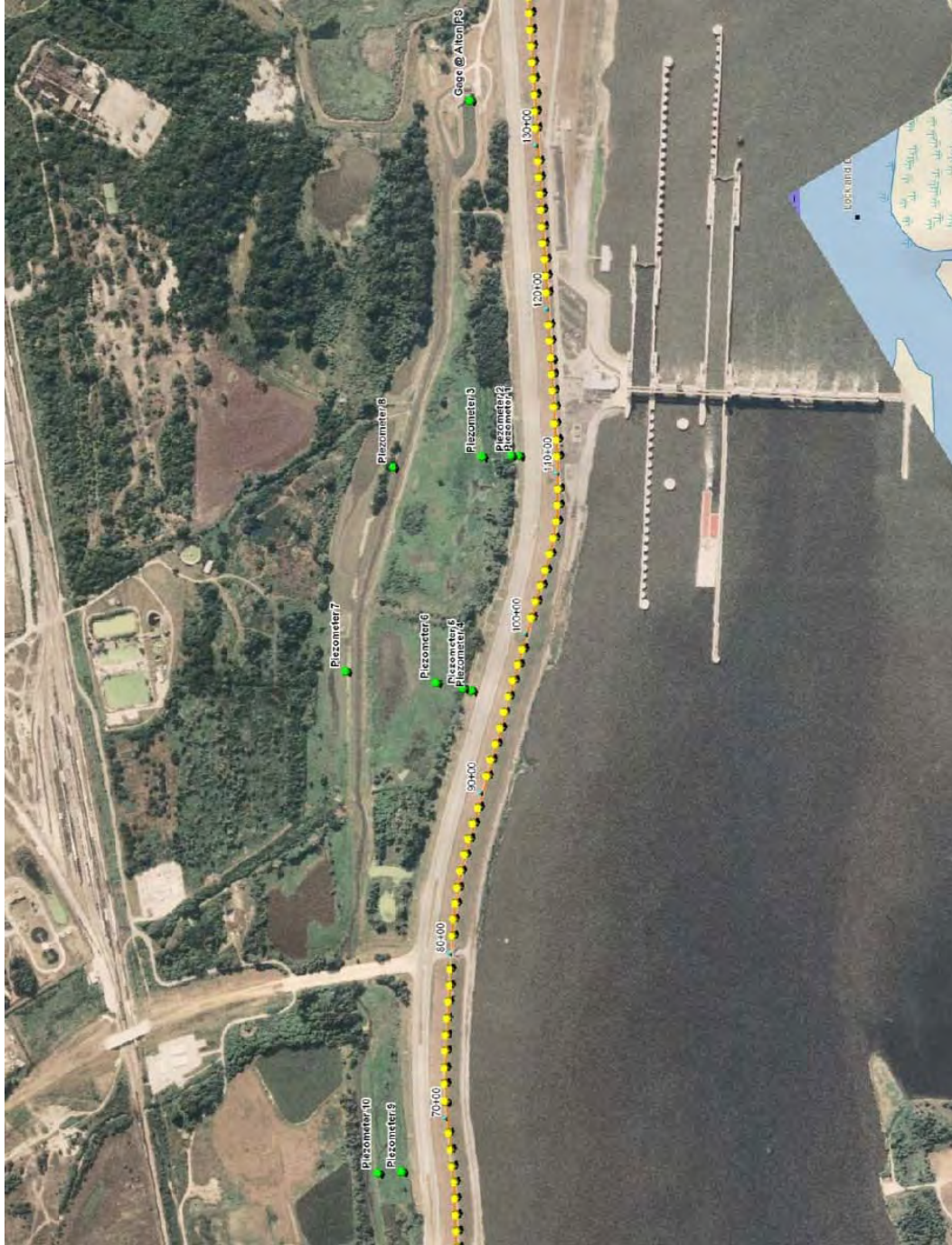
Figure 5.1 – Piezometer Locations (Relief wells not shown for clarity)
