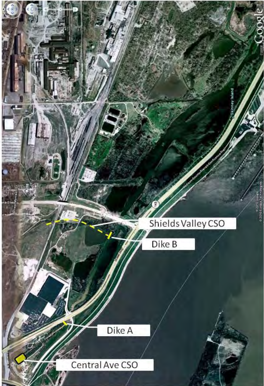
Figure 5.2 – Locations of CSO Structures and Temporary Dikes A & B
