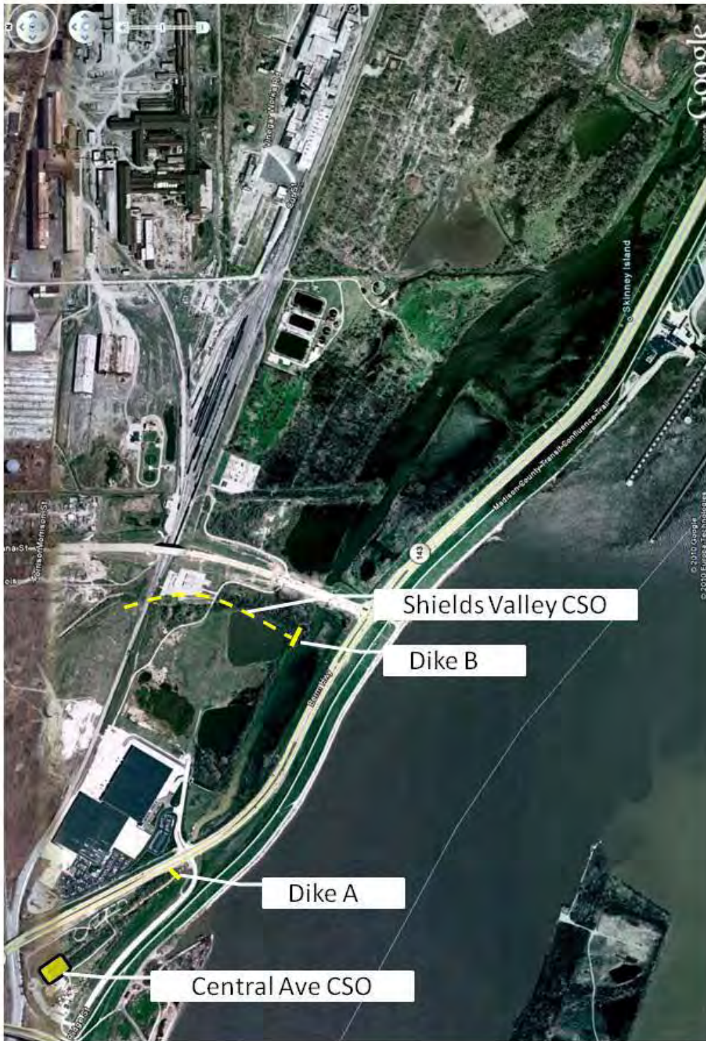
Figure 2.12 – Locations of CSO Structures and Temporary Dikes A & B
