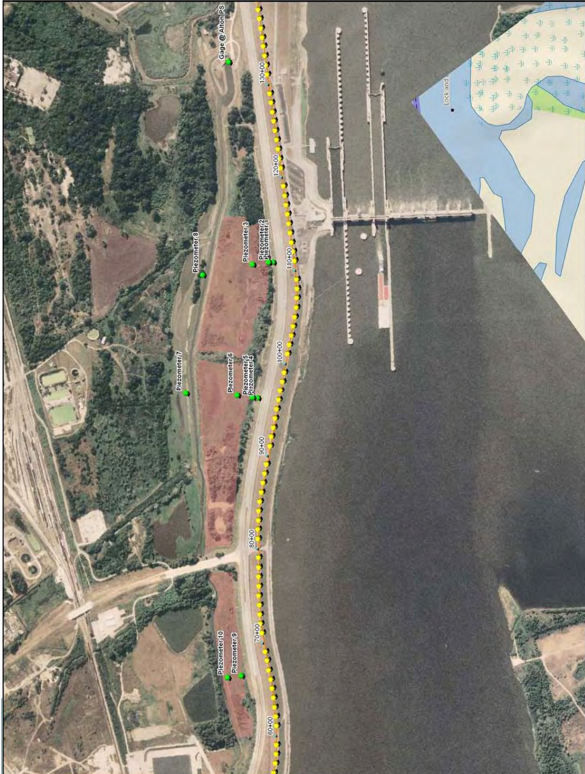
Figure 2.4 – Piezometer Locations and Extents of Serious Seepage Area (Relief Wells and Stationing not shown for clarity)
