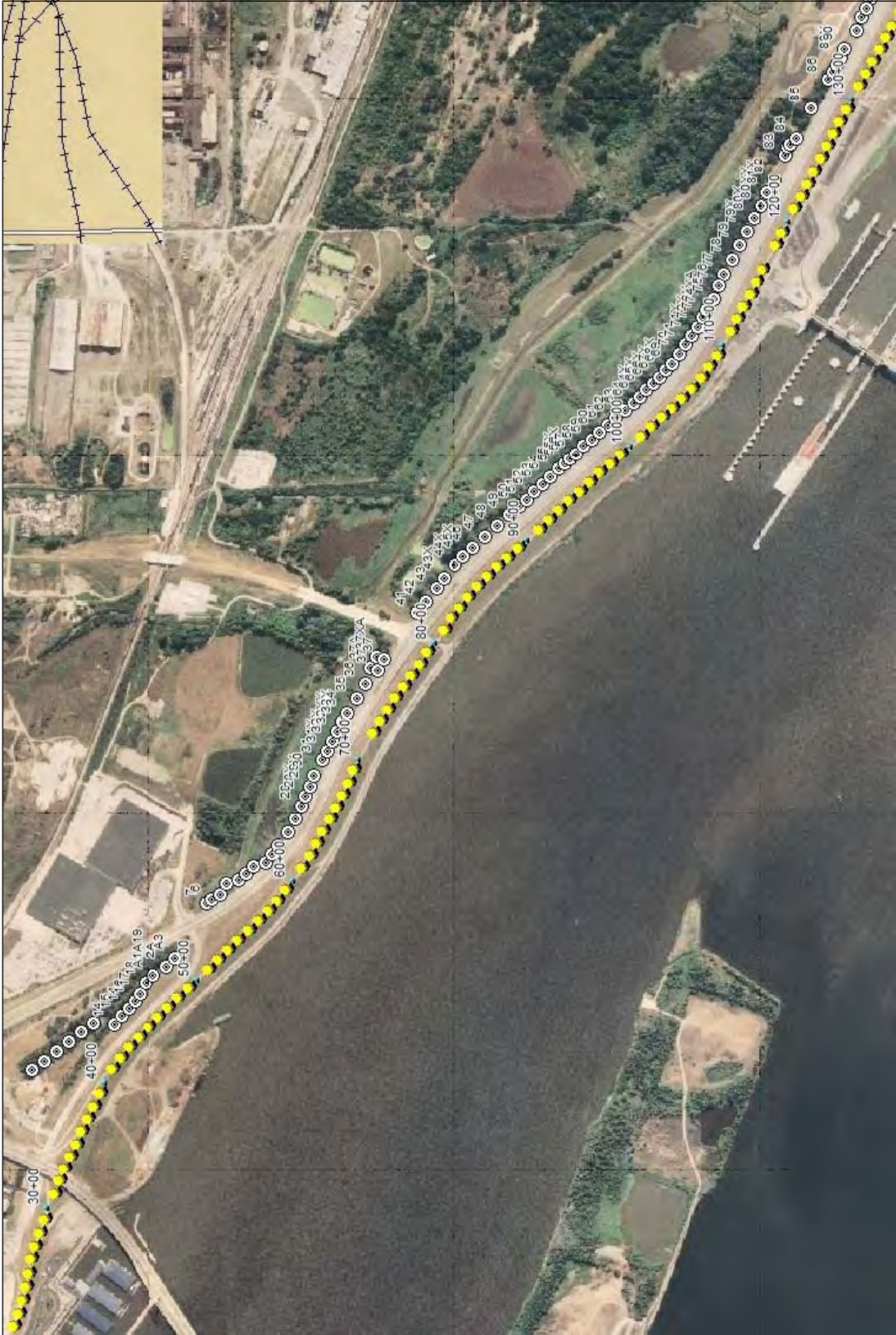
Figure 2.2 – Area Landside of Wood River Levee. Subject of DM-16 Report. (All existing relief wells superimposed on aerial image.)
