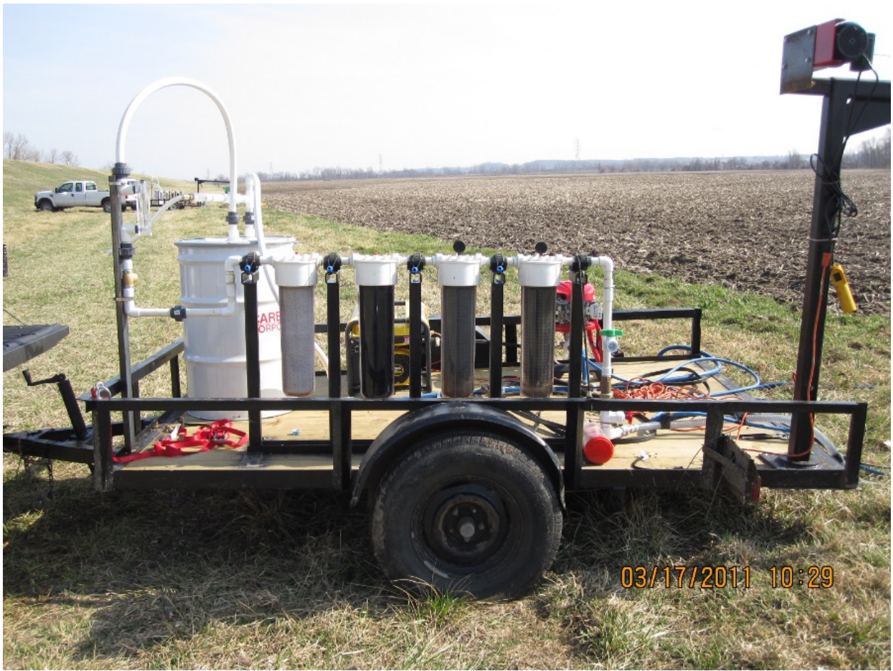
Figure 5: Carbon Filtration System
