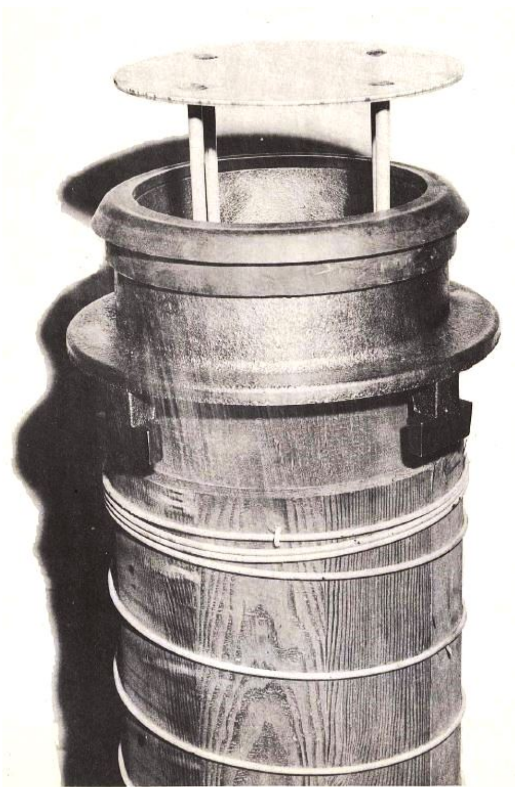
Figure 3: Top to Bottom: Aluminum Check Valve, Rubber Gasket, Cast Iron Tenon, and Wood Stave Relief Well Pipe. (photo credit: USACE)
