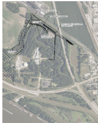
Jack-and-bore 72" RCP under IL-3 Utilities not fully known Considered a betterment (not cost-shared)
